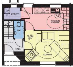
GROUND FLOOR LAYOUT HOUSE TYPE A 2 BED / 3 PERSON HOUSE Ground Floor Area = 34.6m² Total Gross Internal Floor Area = 71.1m²
