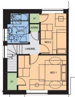
FIRST FLOOR LAYOUT HOUSE TYPE B 2 BED / 3 PERSON HOUSE First Floor Area = 39.2m 2
