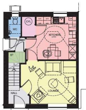
GROUND FLOOR LAYOUT HOUSE TYPE B 2 BED / 3 PERSON HOUSE Ground Floor Area = 39,2m 2 Total Gross Internal Floor Area = 76,4m 2
